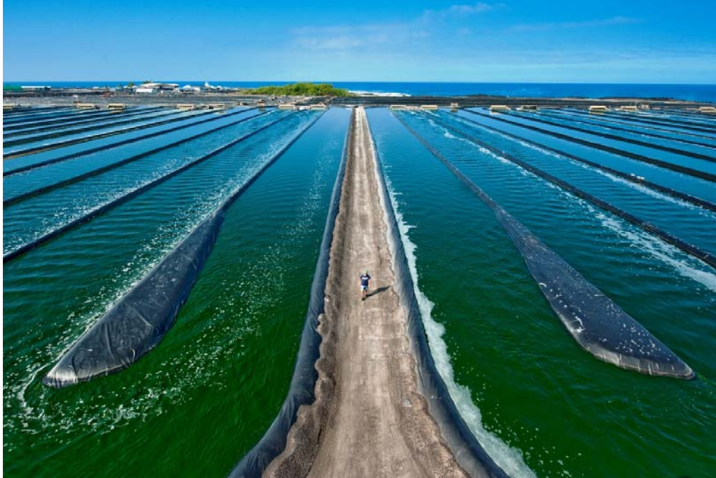
Figure 5. An open-raceway pond designed for the growth of wild-type Spirulina pacifica . Source: Nutrex Hawaii.
