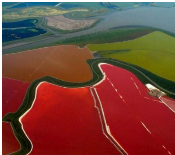
Figure 7. Salt evaporation ponds outside San Francisco. Pond salinity levels can be distinguished by the different cyanobacterial species that grow in them. Containment is provided by levees surrounding the ponds.
