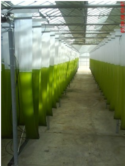
Figure 6. Example of a photobioreactor facility for producing algae and cyanobacteria. Photo from a South African biofuel project. www.saaea.blogspot.com
